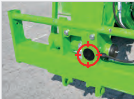
Sensor on the carriage
