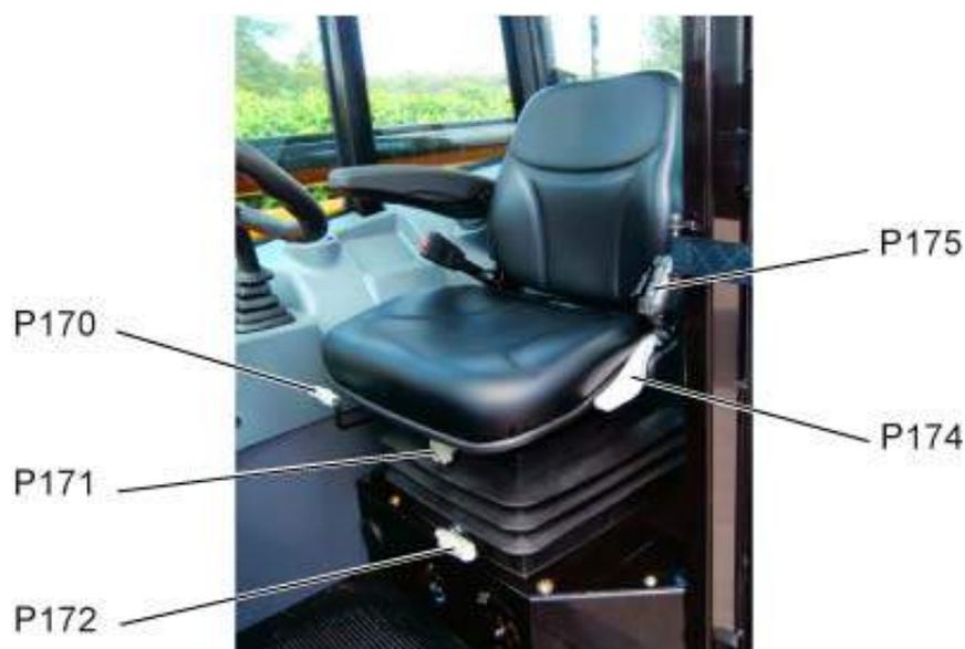
Before starting the engine, adjust the seat as follows to place the seat in an appropriate and comfortable position :
