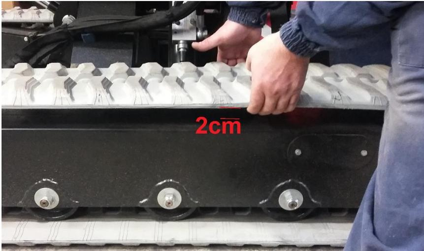
Pull the track slightly upwards in correspondence with the centre line; the deformation must be of approximately 2 cm.
