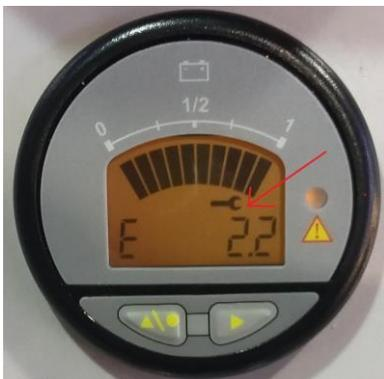
The control unit can store up to 16 alarms which are shown by pressing the right button of the hour counter.
