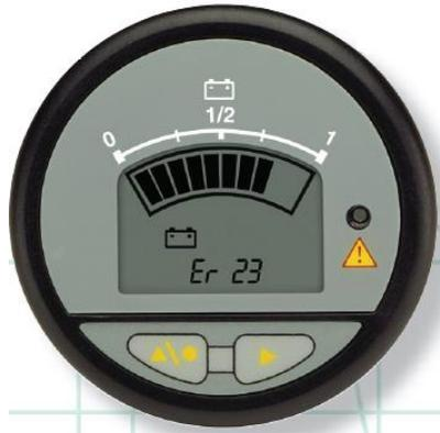
The hour counter, placed next to the ladder, allows to display the machine status. This display also shows any errors and/or alarms that may occur.
