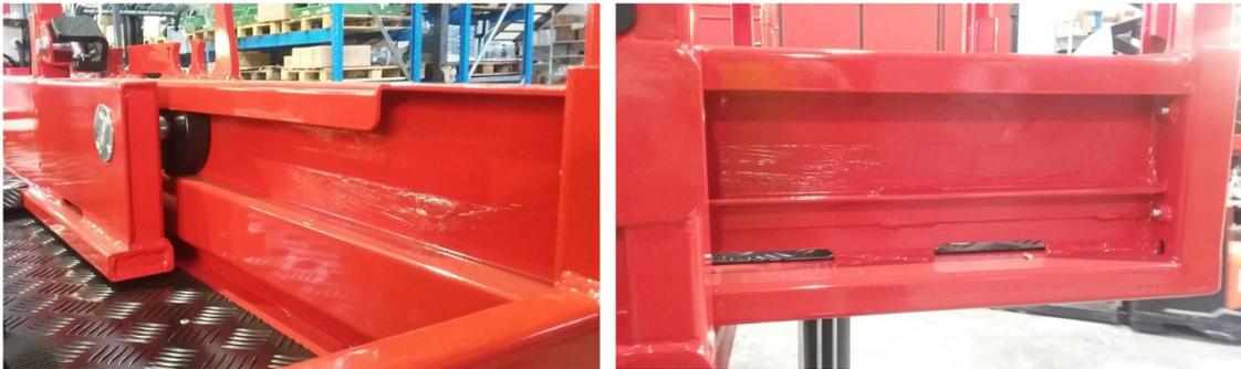
Remove all dirt from the parts before greasing.
