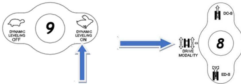
Warning: If selector 8 is positioned on DC-S, the function is not active.
