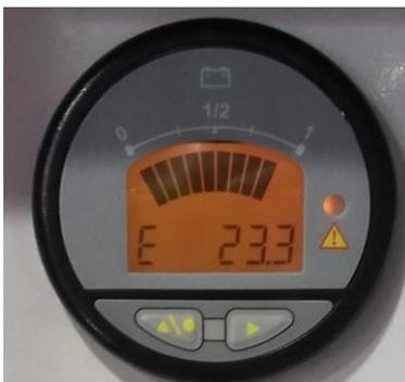
E = hours of operation with electrical engine
