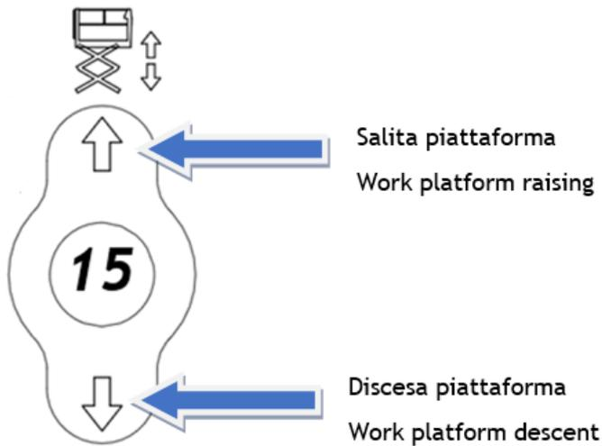
During the downward movement, the ANTI-CRUSHING function is activated, to prevent accidents to the operators on the ground near the machine.
