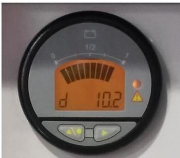
d = hours of operation with diesel engine
