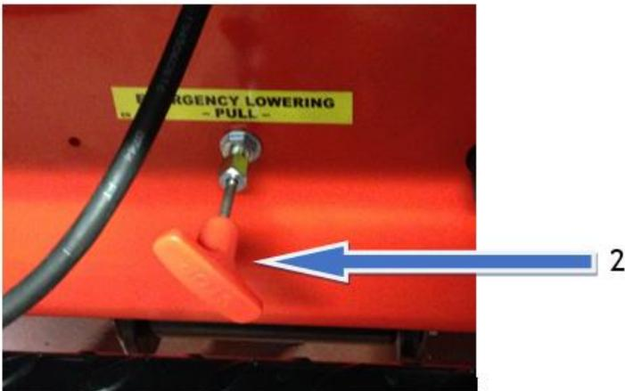
**Warning:** This mechanism must only be used in an emergency, i.e. electrical or hydraulic failure.
