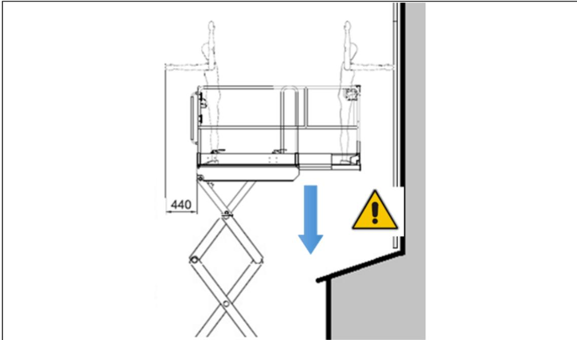
Warning: while descending from the working position, pay warning to possible obstacles beneath the work platform to prevent the platform from overturning or being damaged!
