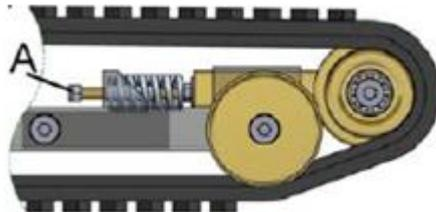
7- Move the front wheel back by pressing on the track with your foot
