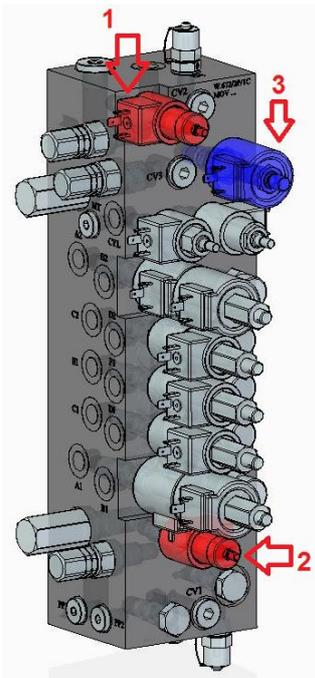
**WARNING: If valve 3 is not reset in the fully activated position by pressing and turning it clockwise (you will hear a click) and valves 1-2 are fully unscrewed (replace the lead seal), the safety of the machine is compromised and the platform may overturn.**
