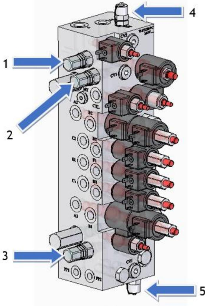
To test them, connect two pressure gauges with a full scale of 250 bar to the pressure outlets supplied (4 and 5).
