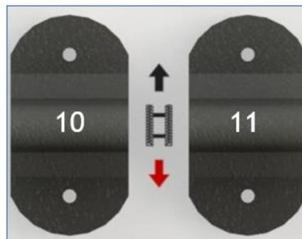
Each lever controls the respective track (right lever→right track, left lever→left track).
