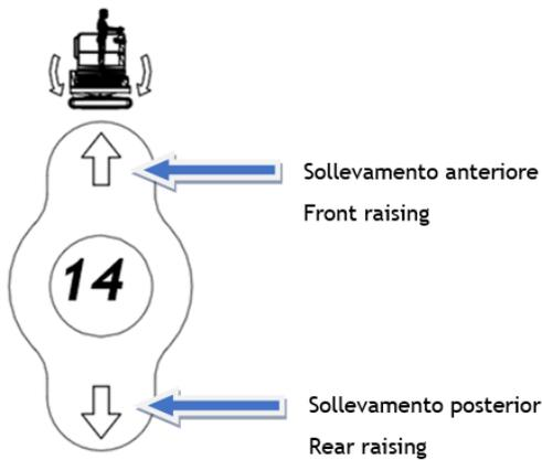
By activating any movement, the platform will stop automatically once it reaches the horizontal.
