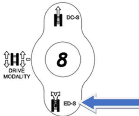
In fact, the activated function controls, in addition to the selected track, also the movement of the other track but at a lower speed.
