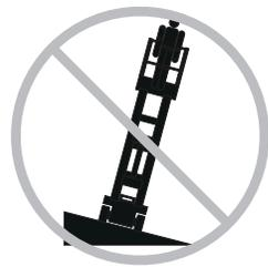
Do not depend on the tilt alarm as a level indicator. The tilt alarm sounds inside the battery charger tray only when the machine is on a severe slope.
