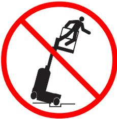
Use extreme care and slow speeds while driving the machine in a stowed position across uneven terrain, debris, unstable or slippery surfaces and near holes and drop-offs.
