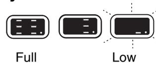
Use the LED diagnostic readout to determine the battery level.
